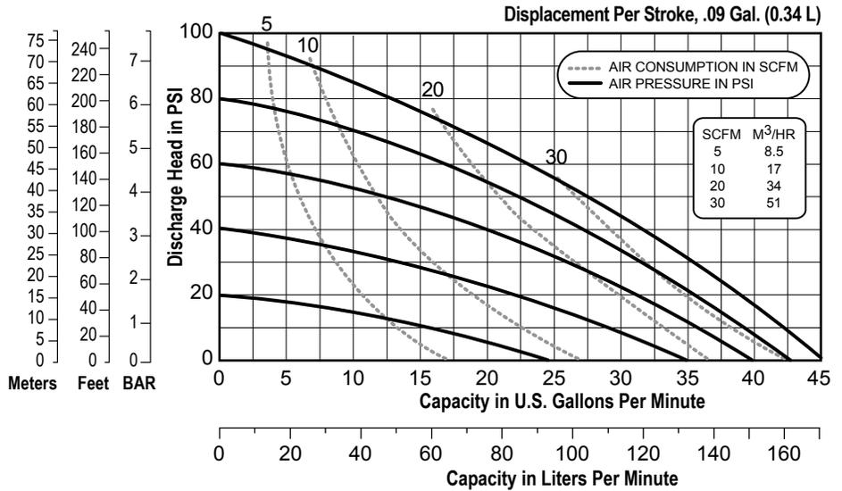
NOTE: Performance based on the following: elastomeric fitted pump, flooded suction, water at ambient conditions. The use of other materials and varying hydraulic conditions may result in deviations in excess of 5%.
